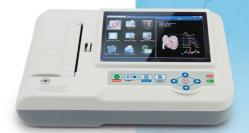
ECG600C six channel ECG is such a kind of electrocardiograph, which sumple I leads ECG signals simultaneously and prints out the ECG waveforms with thermal printing system. Its functions are as follows: Recording and displaying ECG waveforms in auto/namual mode, Auto-measuring and auto-diagnosing the ECG wave parameters. Prompting the state of lead off and paper lack; Switching several kind of interface languages: Managing the case database.
